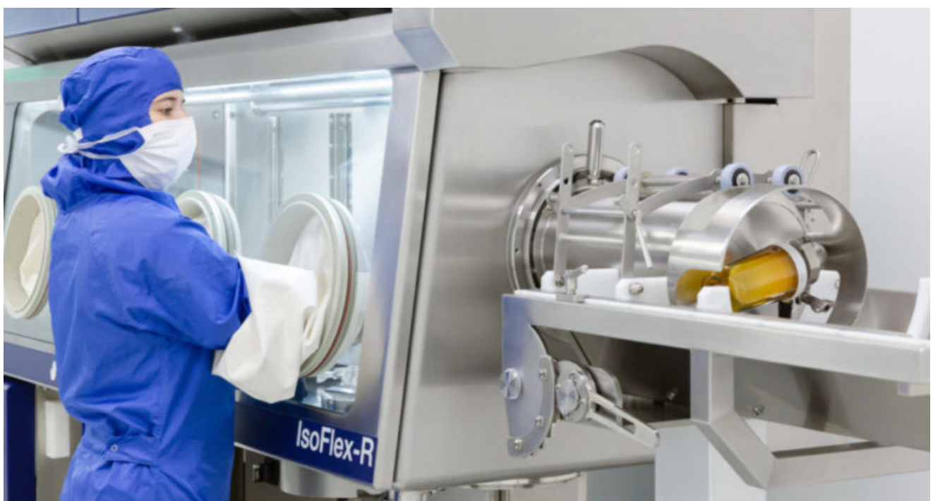
DPTE® Alpha port standard diameters: 105, 190, 270, 350, 460
