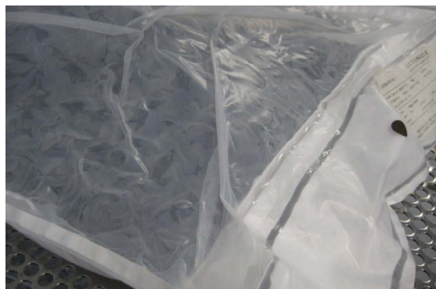
Image 14: Outer and inner bags of the DPTE-BetaBag® double bag, stuck together due to partial film melting (excessive temperature)
