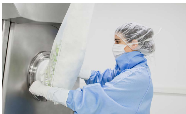
Image 2: DPTE-BetaBag® Tyvek® Ø190 docked to a DPTE® Alpha port
