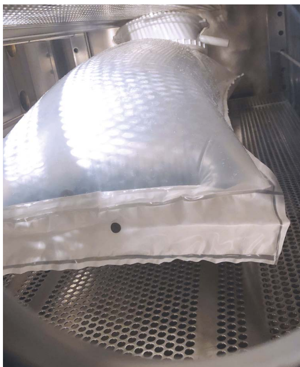
Image 11: Inflation during pressure decrease. Image shows the contact between the DPTE® Beta part and shelf above
