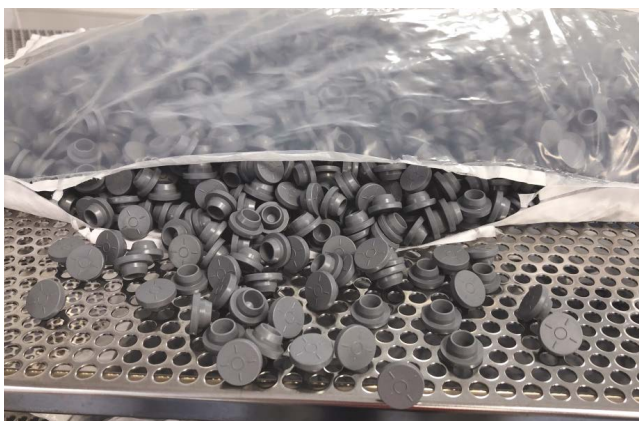
Image 13: Bag welding has peeled due to bag overloading
