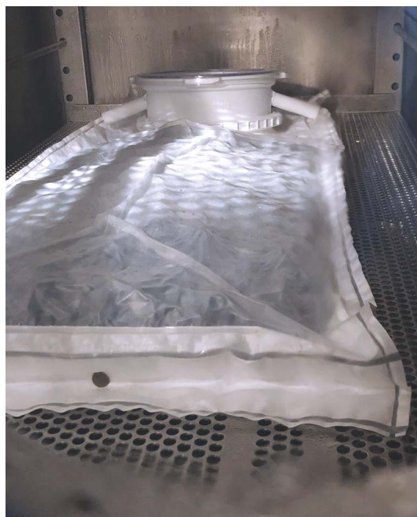
Image 12: Deflated bag during pressure increase
