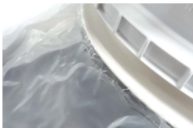
Image 16: Critical film elongation at the connector edge due to HDPE side positioning and/or excessive vacuum ramp
