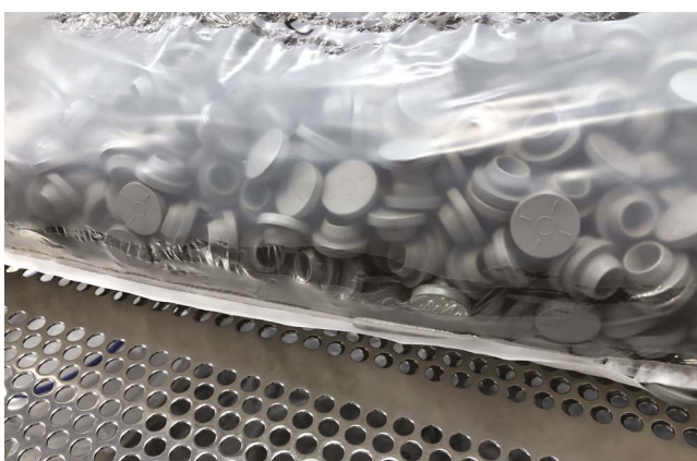
Image 15: Critical film elongation due to bag overloading and/or excessive vacuum ramp
