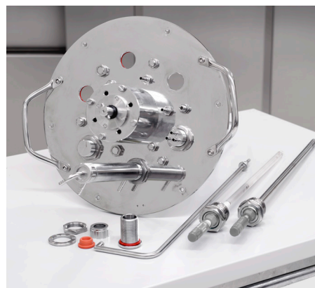
Bioreactor headplate components can be prepared differently for new or repeat applications.
