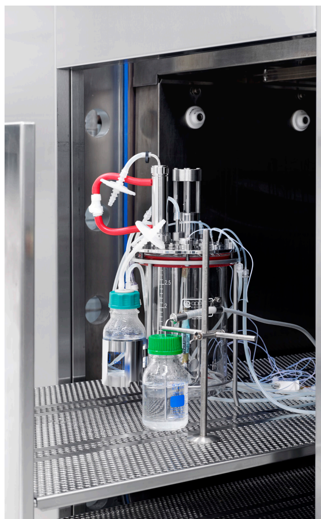
Once the bioreactor and associated components are cleaned, a programmable sterilizer cycle assures final preparation in compliance with protocols essential for validation.
