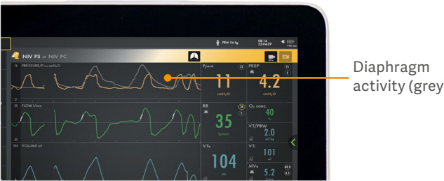
Figure 5 Figure 5 shows how the electrical activity of the diaphragm in grey overlays the pressure curve (yellow), making it easy to see differences in what the patient requests and what the ventilator delivers.
