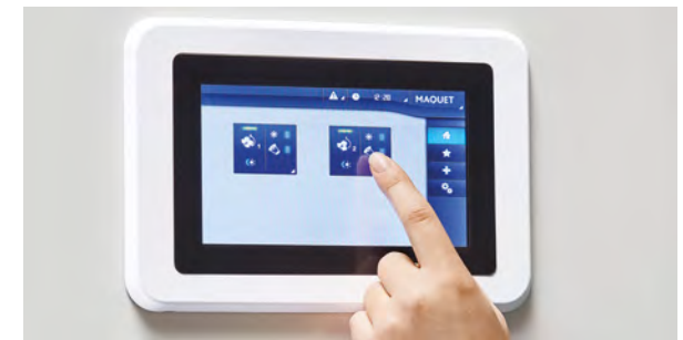
Wall control touchscreen panel
