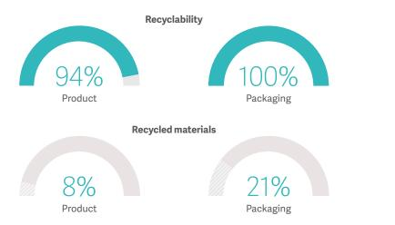
The following materials are considered recyclable: Steel, Alu, Bronze, Brass, Copper (except cables), Cardboard, Paper, Thermoplastics (PMMA, PVC, ABS, PC, PS, PET, PE, PA, PP, POM). Thermosetting plastics, elastomers and other materials not listed are considered non recyclable. Recycled content evaluated in the study but requires documented trail in the value chain.
