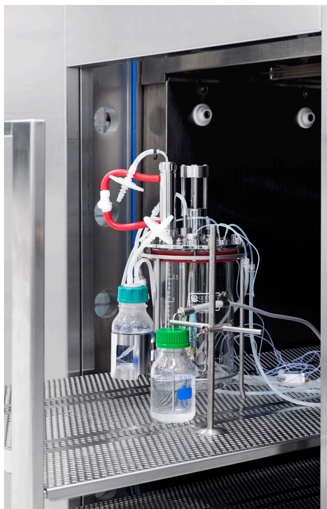
Once the bioreactor and associated components are cleaned, a programmable sterilization cycle assures final preparation in compliance with protocols essential for validation.
