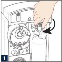
1 Fully close helium tank valve clockwise.
