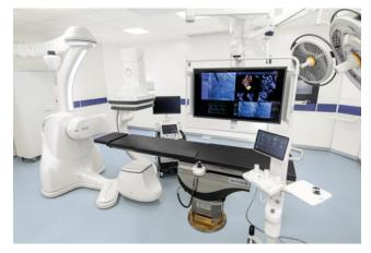
The carbon-fiber table top is ideal for catheter-based or minimally invasive procedures.
