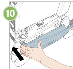
10 Slide helium tank drawer in and replace helium tank panel.
