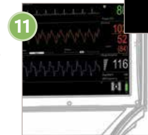
11 Verify full helium level via icon on Monitor Display.
