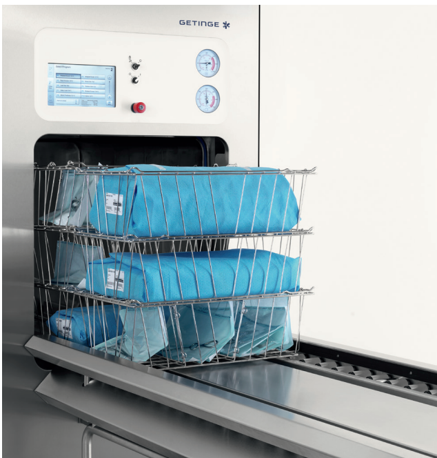
Automatic loader and unloader for baskets (GL64B).
