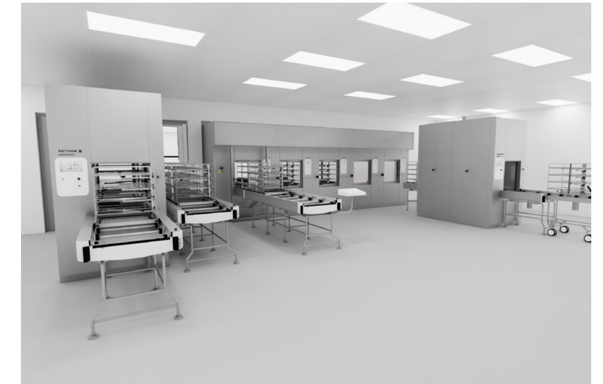
Aquadis Index in combination with AGS and automatic Aquadis Pre-Cleaning Ultrasonic (PCU)
