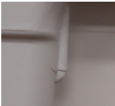
Example for a crack in intellipack packaging tray
